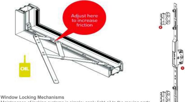
Maintenance of locking systems is simple: apply light oil to the moving parts twice a year. Similarly, a little grease should be applied to the locking keep slots a facilitate smooth running.
