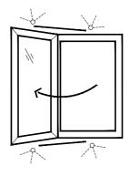
Do not force the sash past the max opening on the hinge or restrictor.
